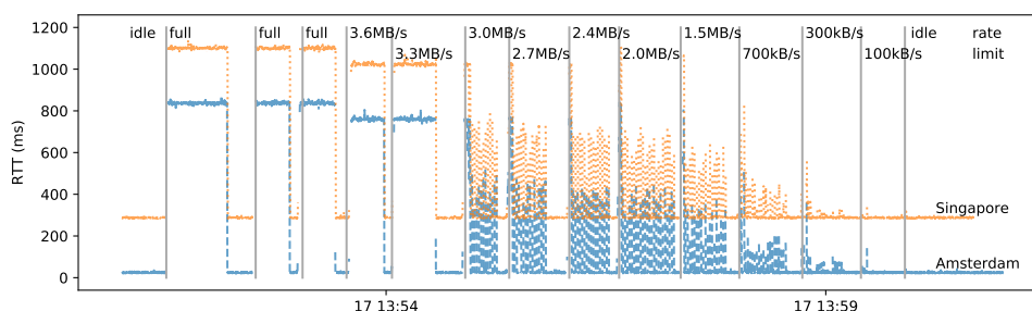
Figure 17: RTT time series from Amsterdam and Singapore toward a typical residential cable access network in Zürich with a 30Mbit download link, during downloads from that network with various rate limits.
